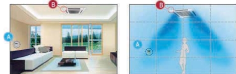
• Temperature setting (A): Indoor unit temperature setting • Temperature setting (B): Wired remote controller temperature setting
