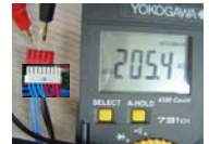
(Example) OLP sensor/discharge temperature sensor measuring resistance value by temperature: E320, E251.
