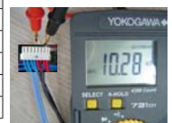
(Example) OLP sensor/discharge temperature sensor measuring resistance value by temperature: E320, E251.
