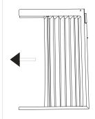
1.Place unit on floor, a bench or a table. Hold the Accordion Panel in one hand and gently pull back the center to free the open end. See Fig.1
