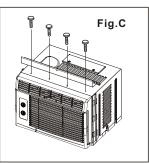
**NOTE:** For safety reasons, all four(4) screws MUST be securely fastened.
