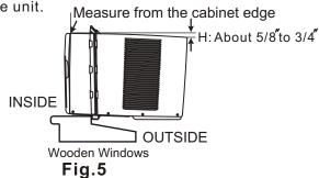
**NOTE:** Check that air conditioner is tilted back about H (Fig.5)(tilted about 3° to 4° downward to the outside). After proper installation, condensation should not drain from the overflow drain hole during normal use. Correct the slope otherwise.
