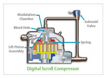
The Copeland Scroll Digital operates in two stages - the "loaded state", during which the solenoid valve is normally closed and "unloaded state", during which the solenoid valve is open. During the loaded state, the compressor operates like a standard scroll and delivers full capacity and mass flow. However, during the unloaded state, there is no capacity and no mass flow through the compressor.
