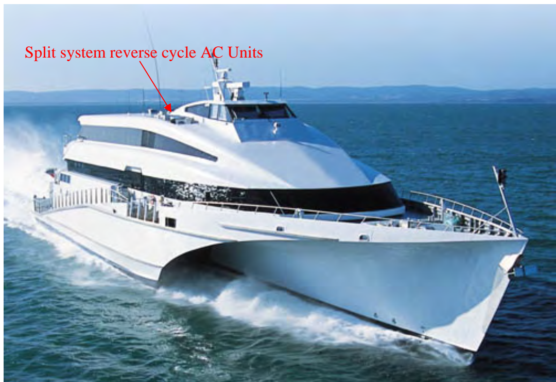
Figure 1.2: A Roof mounted distributed HVAC system as used by Northwest Bay Ships.
