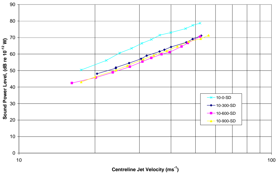
Figure 5.71: Sound power level comparison for the 10° conical diffuser fitted with the square (SD) outlet grill with an extended outlet duct of 0, 300, 600 and 900 mm.
