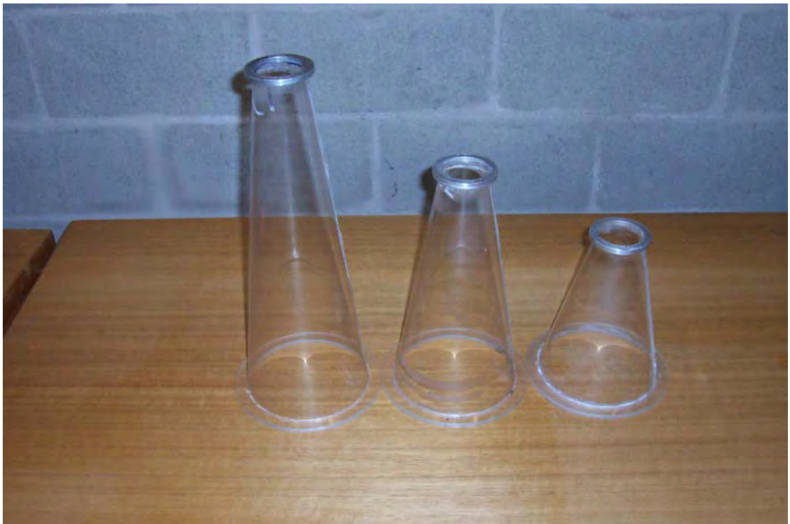
Figure 4.4: The three conical diffusers with an angle of 7°, 10° and 14° (left to right).
