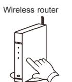
**6** Confirm that LED 2 is flashing. (On/off at 2-second intervals.) Then press and hold the Setting button on the WLAN adapter for 3 seconds.
