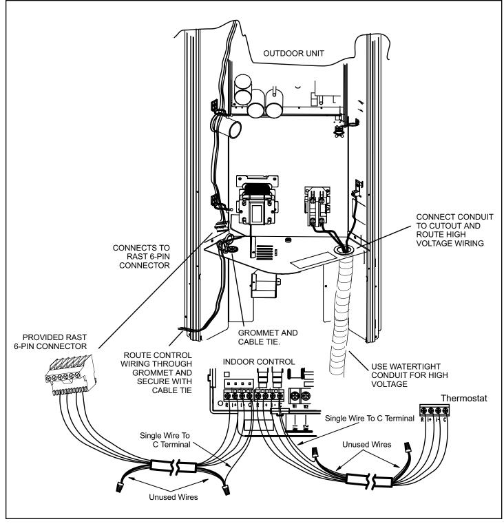
Figure 7. Control Wiring
