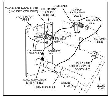
Figure 3. Remove Existing Expansion Valve (uncased coil shown)
