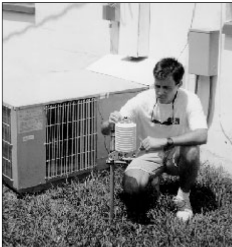
Figure 2. A Research Engineer Adjusts a Pyranometer Leveling Base on the Apparatus Used in the Measurement of Condenser Air and Insolation Conditions at Site 2 (Left); Example of Roof Top Meteorological Station (Right)
