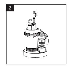
2. Install a check valve (not included) into the pump (or adapter if using 1-1/4 in. pipe).
