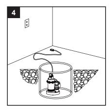
4. Place the pump in the sump, make sure that nothing interferes with switch operation.
