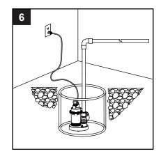
6. Plug the pump into a GFCI outlet.
