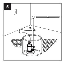
5. Connect the discharge pipe to the other end of the rubber hose, tighten the clamp with screwdriver. **Notice:** A rigid discharge pipe is recommended to prevent the pump from moving. If a flexible discharge hose is used, the pump must be secured in a manner that prevents the pump from moving. If the pump is allowed to move, the float switch could be restricted by the sump wall, preventing the pump from turning on or off.
