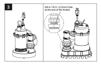
3. Connect a short length (6-10 in.) of rubber hose to the check valve.
