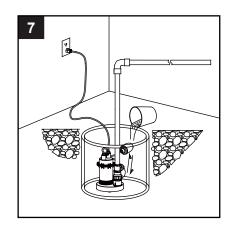
7. Check the pump by filling the sump with water and observe the pump's operation through one complete cycle and make sure the pump cannot move in the sump and float switch moves freely up and down.
