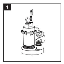
1. Wrap threads of the 1 1/4 in. adapter (included) with thread tape, then screw the adapter into pump outlet hand tight plus 1 turn with a wrench. Notice: If the discharge pipe you will connect is 1 1/2 in., no need to screw the 1 1/4 in. adapter into the pump outlet, just screw a 1 1/2 in. check valve into the pump outlet directly.
