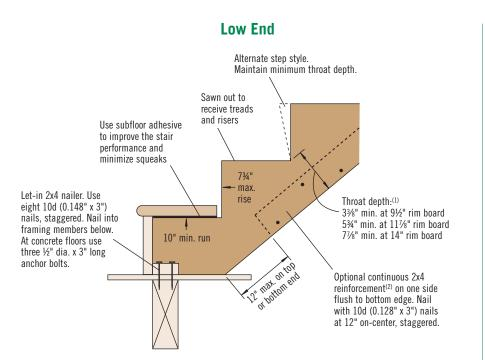
(1) Minimum throat depths may be reduced by an additional ¼" for 11½" and 14" material depths if 2x4 reinforcement is used and provided total rises and runs are limited to table values for unreinforced stringers.
