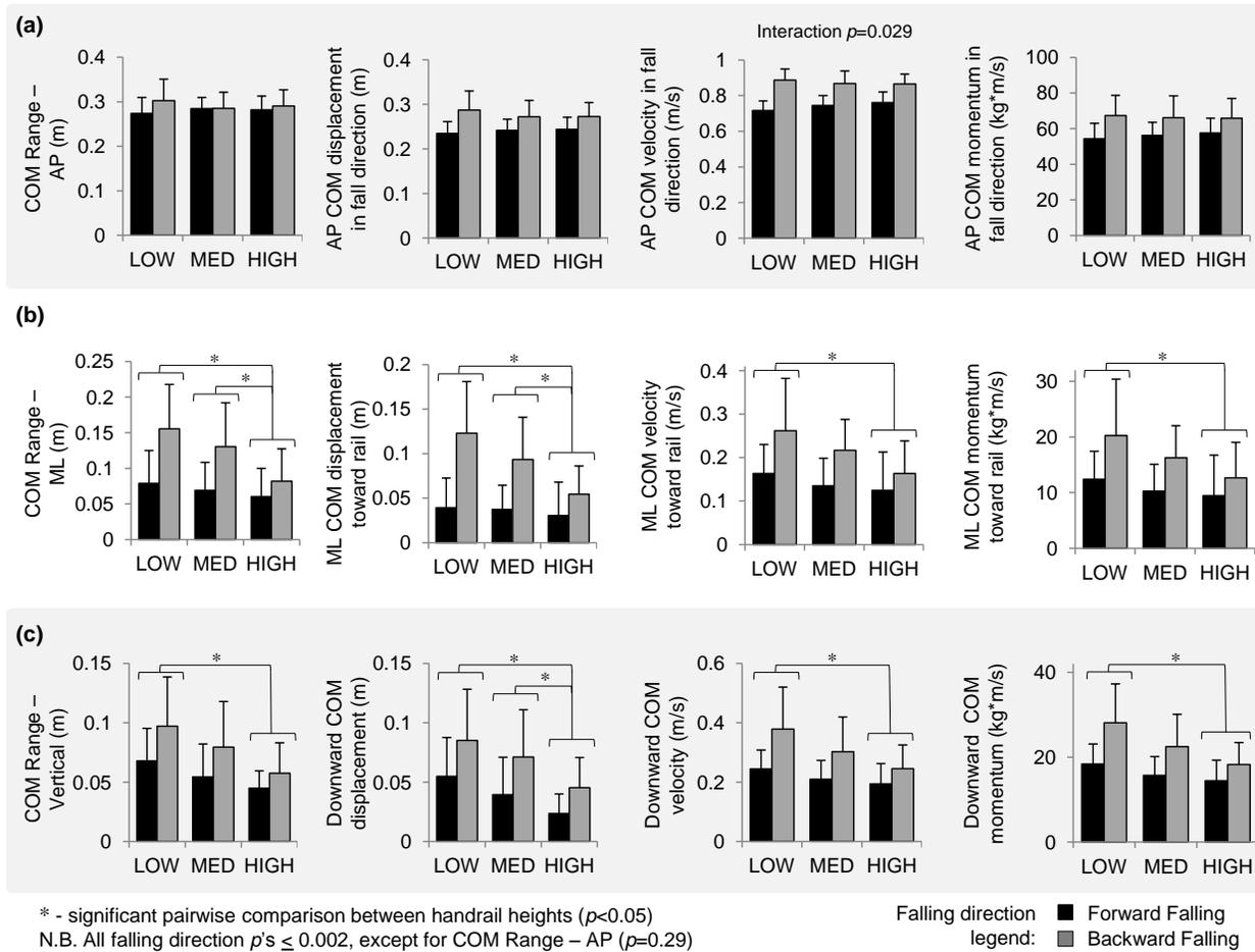
**Figure 4: COM range, and peak displacement, velocity and momentum magnitudes** in the (a) antero-posterior (A-P), (b) medial-lateral (M-L), and (c) vertical axes. Bars represent mean values; error bars represent standard deviation.
