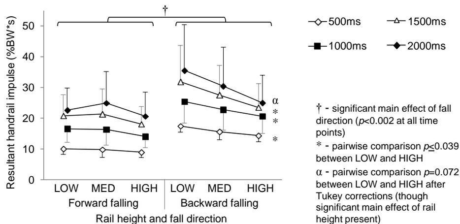
**Figure 3: Resultant handrail impulse for each condition**, measured 500ms, 1000ms, 1500ms and 2000ms after initial handrail contact. Mean values are plotted; error bars represent standard deviation.
