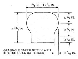
Figure R311.5.6.3(2) TYPE II HANDRAIL
