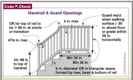
R312.1.2 Height. Required guards at open-sided walking surfaces, including stairs, porches, balconies or landings, shall be not less than 36 inches (914 mm) in height as mea-sured vertically above the adjacent walking surface or the line connecting the nosings.
