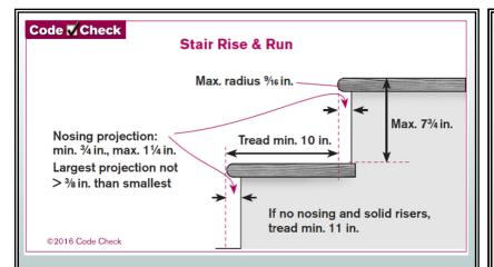
• R311.7.5 Stair treads and risers. Stair treads and risers shall meet the requirements of this section. For the purposes of this section, dimensions and dimensioned surfaces shall be exclusive of carpets, rugs or runners.
