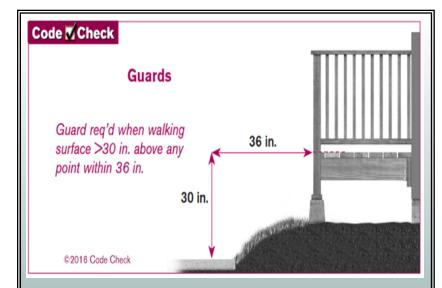
R312.1.1 Where required. Guards shall be provided for those portions of open-sided walking surfaces, including stairs, ramps and landings, that are located more than 30 inches (762 mm) measured vertically to the floor or grade below at any point within 36 inches (914 mm) horizontally to the edge of the open side. Insect screening shall not be con-sidered as a guard.
