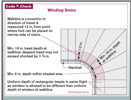
R311.7.5.2.1 Winder treads. Winder treads shall have a tread depth of not less than 10 inches (254 mm) measured between the vertical planes of the foremost projection of adja-cent treads at the intersections with the walkline.
