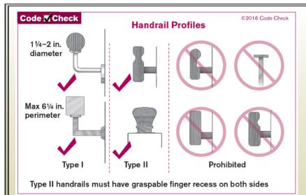
R311.7.8.5 Grip size. Required handrails shall be of one of the following types or provide equivalent graspability.
