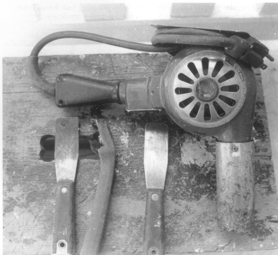
Figure 3. Heat guns, putty knives with corners rounded, and paint scrapers were used in paint removal. Photo: Michael Lee
