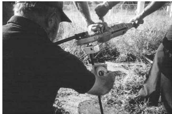
Figure 2.1 Soil test torque probe measures soil bearing capacity for soil classification.
