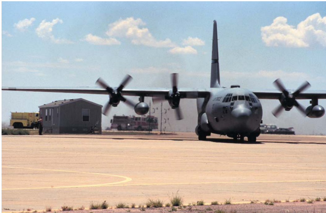
Figure 4.32 May 2001—Texas Tech University, U.S. Department of Energy, and U.S. Department of Housing and Urban Development “overstressed” a single section manufactured home and its Vector Dynamics foundation with 110 mph windgusts from the propwash of a C130 aircraft in Lubbock, Texas.
