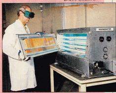
To simulate long-term exposure to sunlight, finish samples were exposed to 90 hours of high-intensity, ultraviolet light in this weatherometer (above). UV exposure yellowed some finishes more than others.
