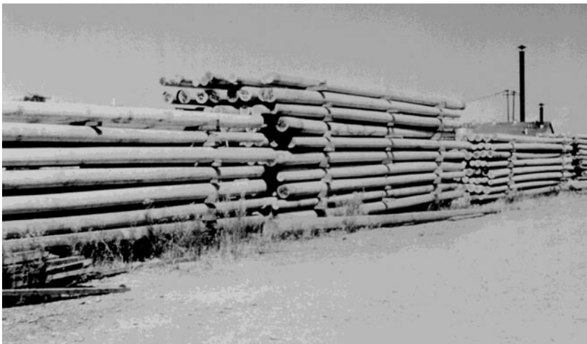
Figure 3. Air seasoning poles.
