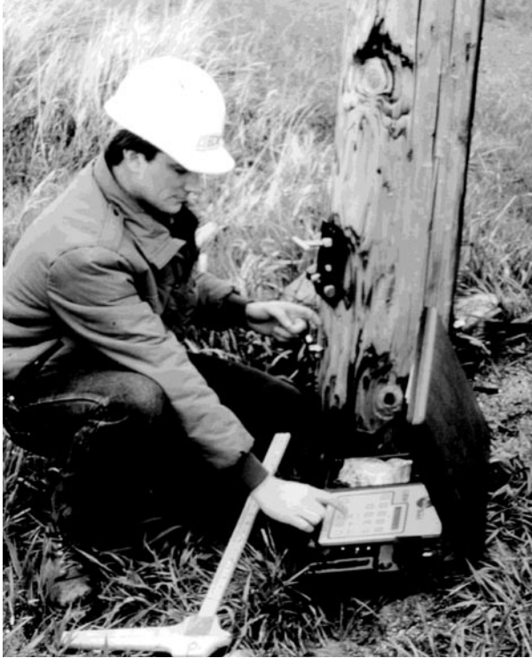
Figure 30. Pole test: an example of an acoustic inspection device.
