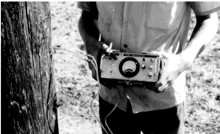
Figure 26. The Shigometer™ measures electrical resistance to detect rot in poles. Use an increment borer to determine the nature of the defect.
