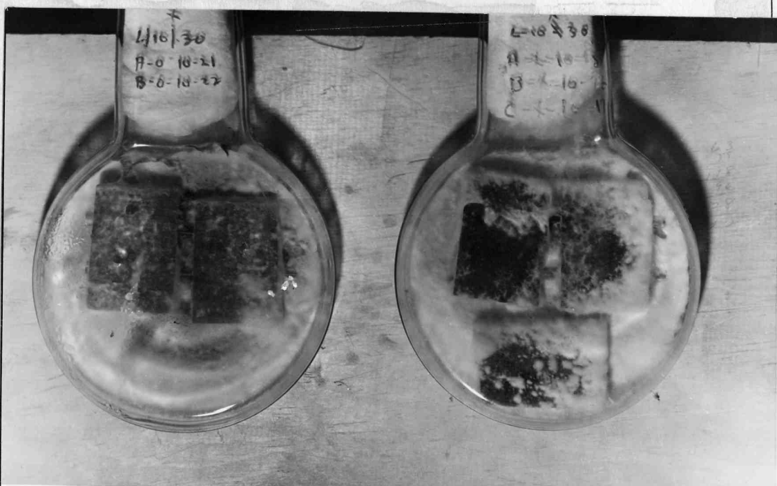
LEACHING TESTS ON BLOCKS TREATED WITH 10% CREOSOTE Left, Oil tar creosoted blocks 21 and 22. Right, Coal tar creosoted blocks 15, 16 and 17.
