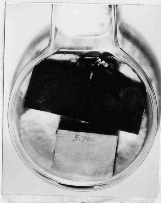
UNTREATED CONTROL BLOCKS ON CULTURES OF LENZITES TRABEA FOR A PERIOD OF 8 WEEKS.
