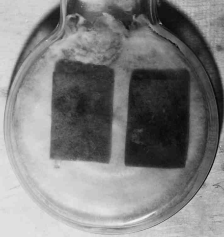
INITIAL TOXICITY TESTS ON BLOCKS TREATED WITH 6% CREOSOTE Left, Coal tar creosoted blocks 9 and 10
