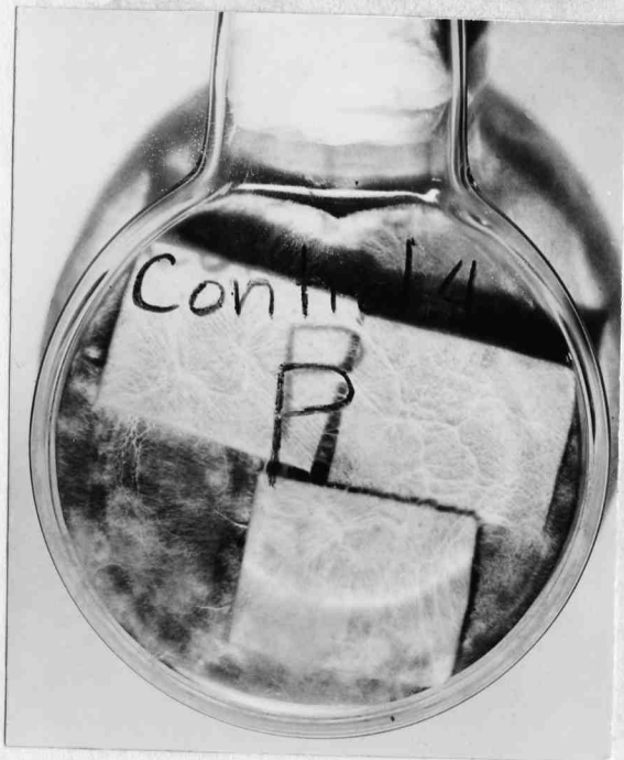
UNTREATED CONTROL BLOCKS ON CULTURES OF PORIA INCRASSATA FOR A PERIOD OF 8 WEEKS.
