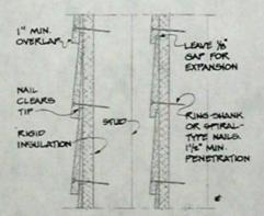
Improper nailing is the most frequently cited cause for wood siding failures over foam sheathing. Use long enough nails but don't nail so hard as to cup the siding.
