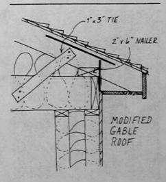
Raising the rafters above the ceiling joists is an easy solution for stick builders.
