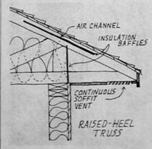
Trusses can be raised with webbing or blocking to make room for insulation.
