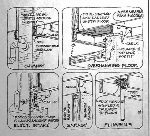
OLD FLOORS CAN BE TRICKY to seal—particularly with board-type subflooring. If the house is built over a vented crawlspace or an unheated basement, the floor should be sealed as well as possible from the prime living space. This limits infiltration and keeps moisture and radon (if present) out of the living space. If the basement is finished and heated, it is usually sealed at the walls, not at the floor above.
