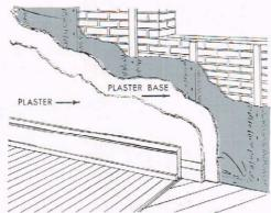
SIDEWALL: Solid Brick or Concrete Block:
