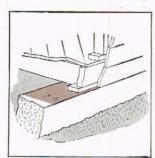
(See illustration at left): 2-oz. or 3-oz. Copper Armored Sisalkraft protects sills and joists against rotting caused by moisture rising through foundations. In the average home this would cost about \$15.00 for 2-oz., or about \$20.00 for 3-oz. Copper Armored Sisalkraft.
