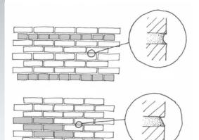
Above are bonding patterns and mortaring profiles typical of those found in the district. The illustration following demonstrates correct and incorrect removal and replacement of mortar.
