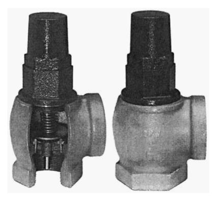
Figure 22 Antisiphon valves are designed to prevent liquid siphoning if piping or fittings below the tank liquid level leak or fail. (Photograph courtesy of OPW Fueling Components.)
