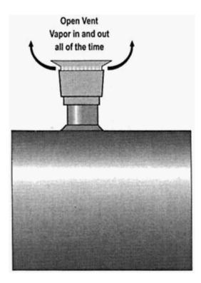
Figure 6 Normal vent-open vent style.
