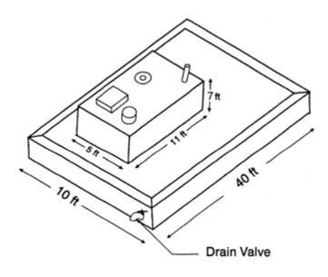
Figure 15 A rectangular 2,000-gal. protected aboveground storage tank.
