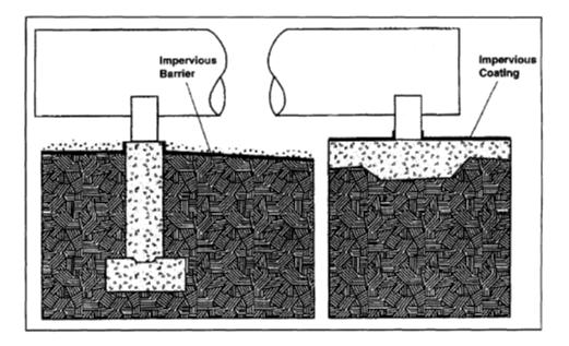
Figure 5 Horizontal tank supports.
