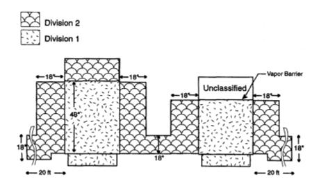
Figure 25 The division 1 and division 2 location boundries for dispensers are specified in NEC® article 514 and UL 87.
