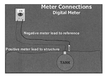
Figure 1 Meter connections: digital meter.
