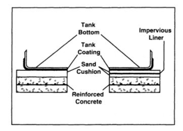
Figure 4 Vertical tank base section.
