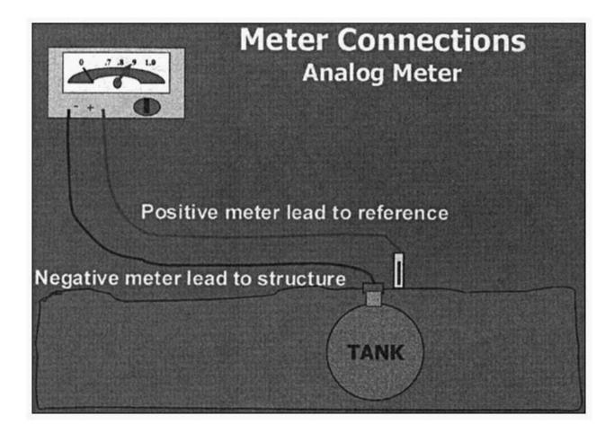
Figure 2 Meter connections: analog meter.
