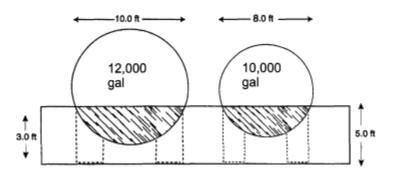
Figure 9 12,000-gal and 10,000-gal horizontal aboveground storage tanks inside of secondary containment.
