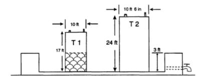
Figure 10 Two vertical aboveground storage tanks.
