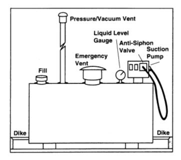
Figure 8 Tank-mounted suction system.
