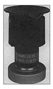
Figure 13 This pressure/vacuum vent is designed to remain closed except when product is introduced or removed from the tank. (Photograph courtesy of OPW Fueling Components.)
