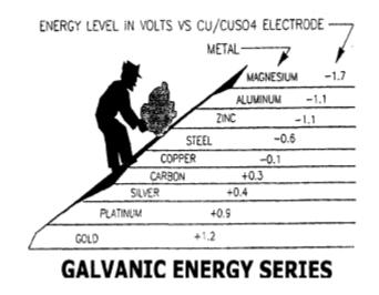
Figure 3 Nature has endowed each metallic substance with a certain natural energy level or potential.
