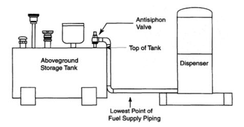
Figure 21 Illustration of AST with antisiphon valve.
