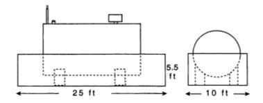
Figure 7 8000-gal horizontal aboveground storage tank located inside of a rectangular secondary containment.
