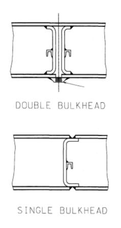
Figure 1 Bulkheads for compartment tanks. Flange for testing may be located anywhere on tank circumference, between two bulkheads.
