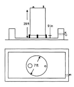
Figure 16 8000-gal vertical aboveground storage tank.
