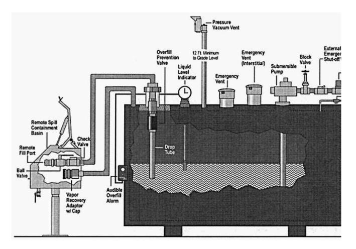
Figure 4 Aboveground fuel storage-pressure system. Rectangular double-wall tank with remote fill and side mounted dispenser.
