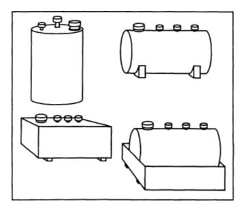
Figure 7 Typical tank profiles.
