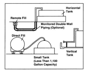
Figure 10 Typical fill methods.
