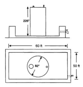
Figure 5 5000-gal vertical tank.
