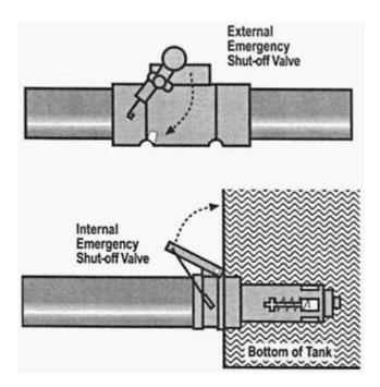
Figure 5 Emergency shut-off valves.
