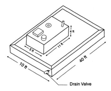
Figure 4 1500-gal rectangular tank.
