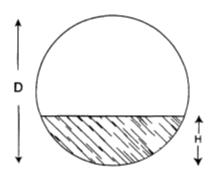
Figure 8 Horizontal tank ullage figure.
