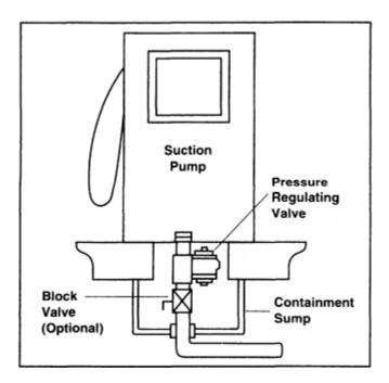
Figure 13 Pressure regulating valve.
