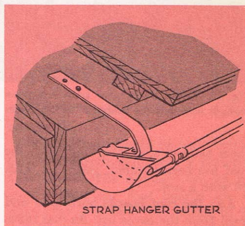
Fig. 26. Gutter hangers should be installed before the roofing is applied and should be nailed to roof sheathing.
