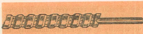
Fig. 27. A single uninsulated wire in an armored cable is used to ground the house electrical system.
