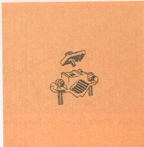
Fig. 28. Ground clamp used to secure ground wire to plumbing line.
