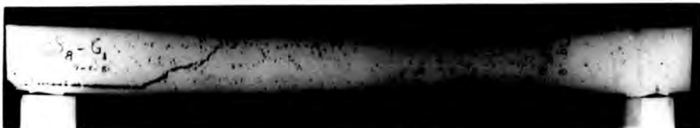
Beam of A_S = 118.0 \text{ mm}^2 (face S_8 ) and core G_1
