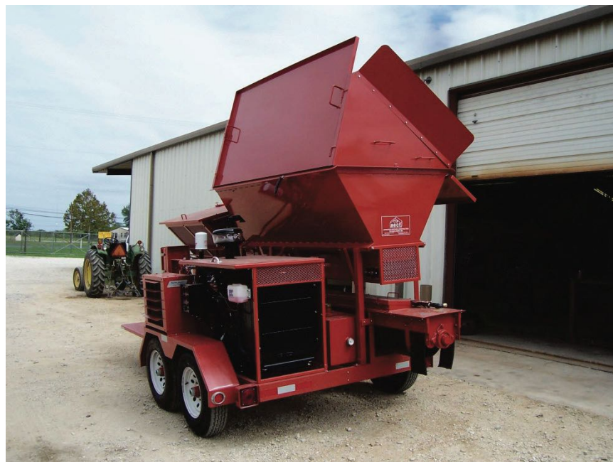
Figure 6. Advanced Earthen Construction Technologies (AECT) MX20 CEB Mixer
