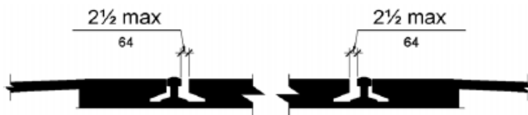
(Exception) Track Crossings
