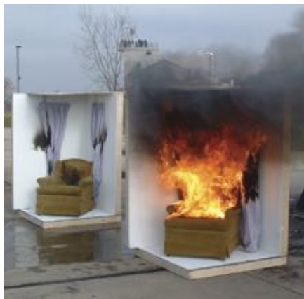
Room-corner burn demonstration for fire-resistive coatings: In the left structure, the chair and drapes were treated with a fire-retardant material and the walls were treated with an intumescent fire-resistive latex paint. The structure on the right was untreated. Photo courtesy of NoBurn Inc.
