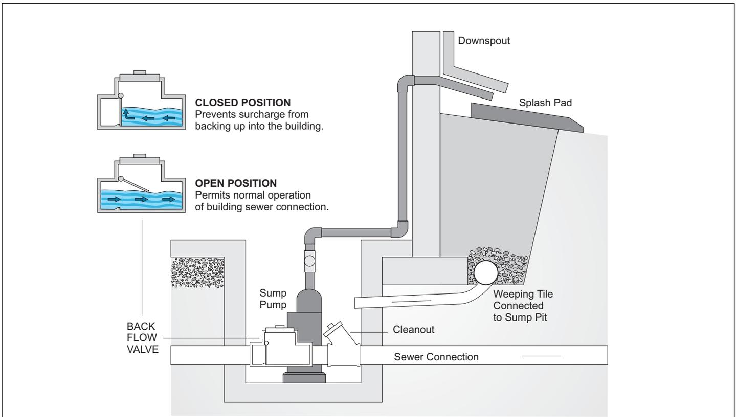
**BACK FLOW VALVES AND SUMP PUMPS ARE EFFECTIVE MEANS OF AVOIDING BASEMENT FLOODING**
