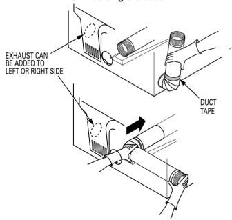
• Apply duct tape as shown on the joint between the dryer internal duct and the elbow.
