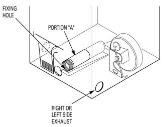
Reconnect the cut portion (A) of the duct to the blower housing. Make sure that the shortened duct is aligned with the tab in the base. Use the screw saved previously to secure the duct in place through the tab on the appliance base.
