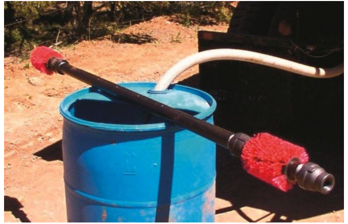
Brush to be attached to drilling rig as one method of physical rehabilitation.
