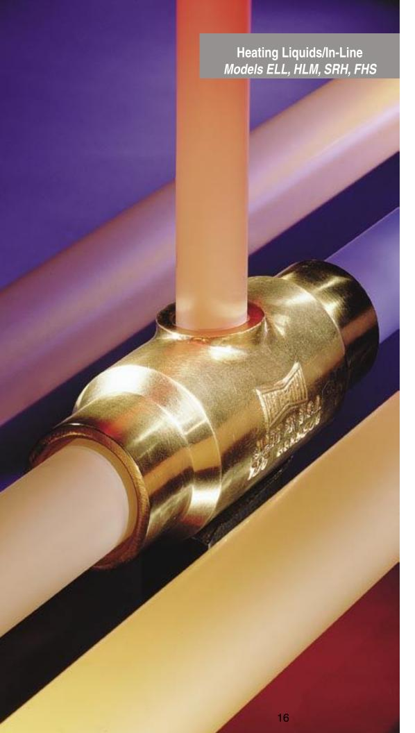
Many process operations can be heated in-line. With Penberthy in-line mixers, you can heat in-line while transporting the process media from one location to another. Steam jet heaters optimize the condensing of steam into the motive media to provide fluid heating. Models ELL and HLM are ejector-type heaters capable of operating at steam pressures lower than the operating liquid. They offer much higher thermal input than a comparable SRH, while incurring a higher inlet to discharge pressure drop.
