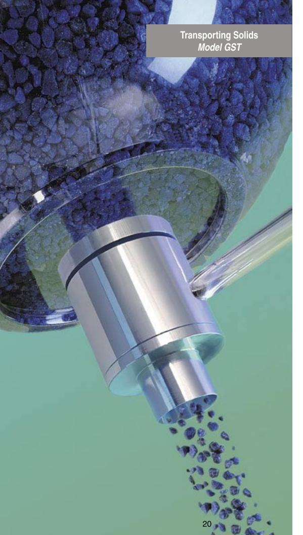
Jet pumps may also be used to transport dry solids using a gas (e.g., air) as its motive source. The Penberthy **Model GST** (gasoperated solids transport) jet pump is designed to pneumatically convey powders and bulk solids via dilute phase through a closed piping system.
