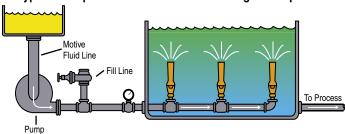
Typical Multiple SCTE Installation For Recirculating Tank Contents
