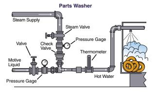
Heating Liquid In-Tank with Model SRH
