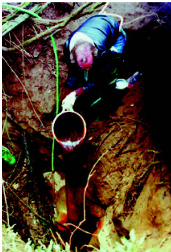
Wellhead protection study. Pouring nontoxic dye for an aquifer time-of-travel test (dye tracing).
