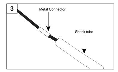
4. Hold a torch approximately 6 in. from the center of the tubing and move it back and forth. Heat one set of wiring tubing at a time until seal is completed. During the heating process, keep all other wires/tubing away from heat to prevent melting together. Avoid overheating, as this may make the tubing brittle. When liquid oozes from end of tube, seal should be complete. (Fig 4)
