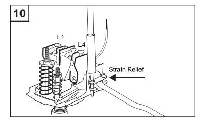
11. Connect the two wires from the house electrical service to the outside pressure switch terminals (L1 and L4). (Fig. 11)
