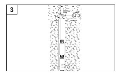
4. Add a well seal or pitless adaptor to allow for the pipe to be connected to house service. (Fig. 4)
