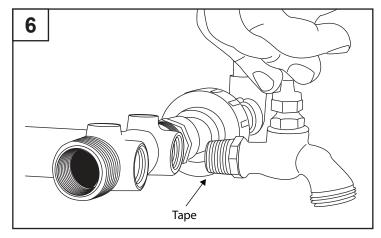
WARNING: Not providing a relief valve can cause extreme overpressure that could result in personal injury and/or property damage.
