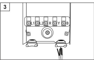
4. Attach the black, yellow and red wires to the appropriate terminals marked "B", "Y" and "R". (Fig. 4)
