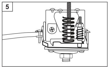
Connect the two wires from the pump to the inside pressure switch terminals (L2 and L3). (Fig. 6)
