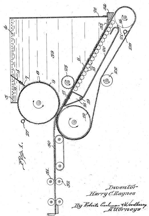
APPARATUS FOR PRODUCING FIBER BOARD
