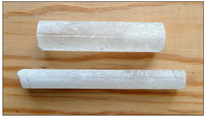
Figure 15. Examples of boron rods that can be placed into holes in cabin logs.
