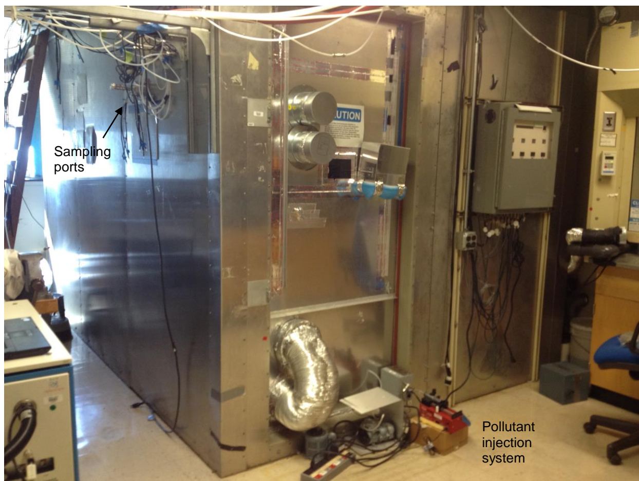
Figure 3.1.1. LBNL's 20-m 3 environmental chamber
