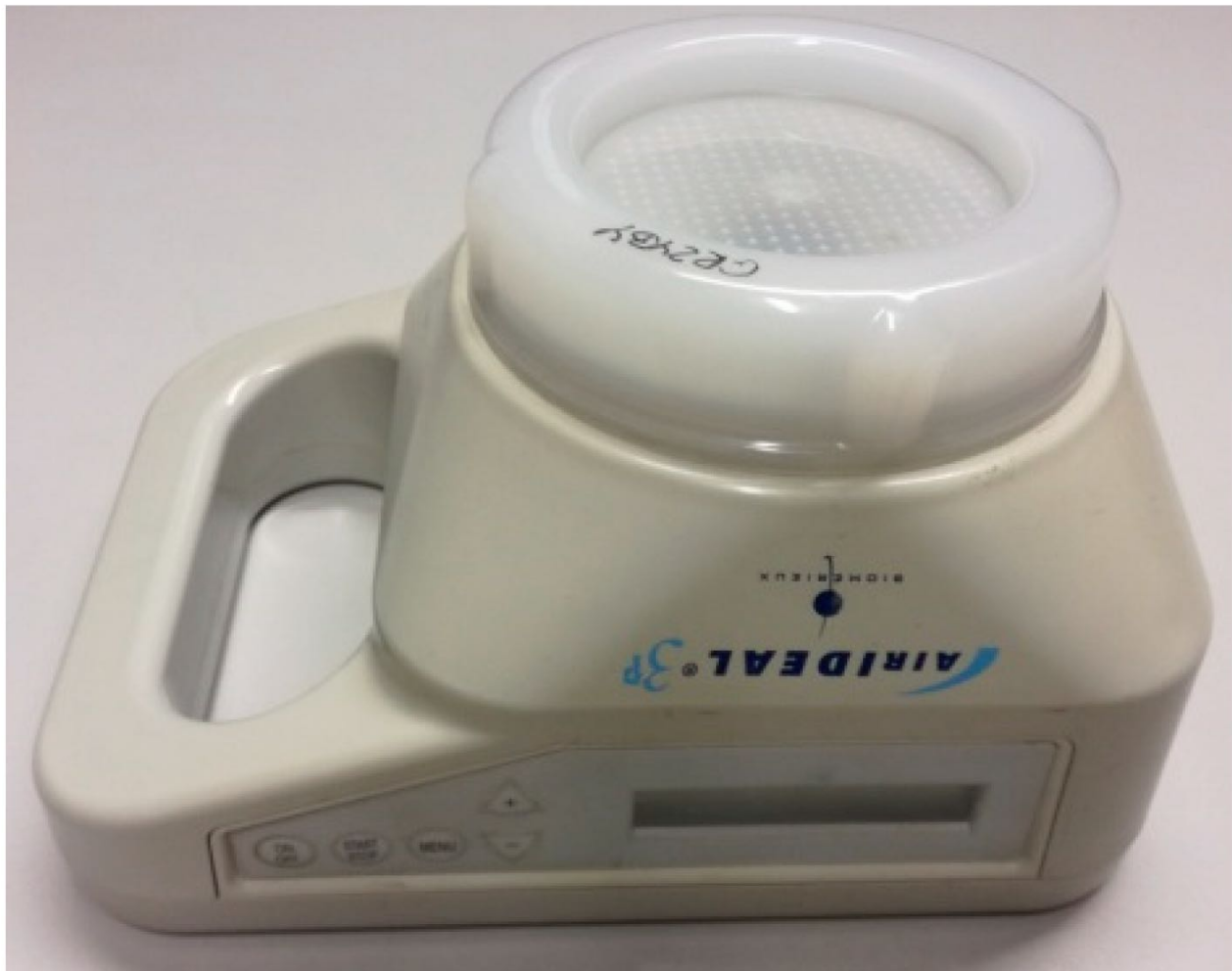
Figure 2. Air Ideal (AI) one-stage impactor used during the study.
