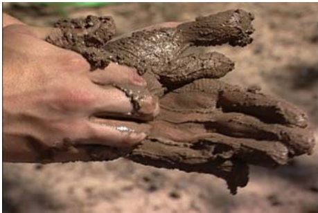
Figure 12. Even soils with significant sand content can smear, it is important to check.
