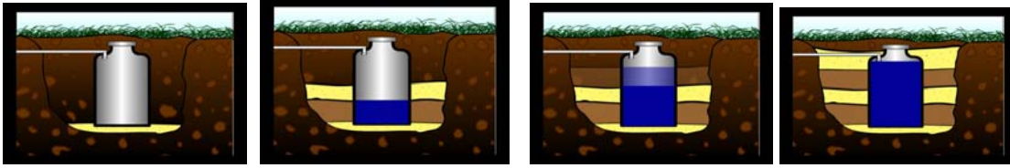
Figure 10. Filling tank and back-filling around tank must be done in sequence of lifts.
