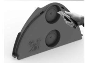
5. Place lip of endcap over the end of the chamber unit and snap into place. Secure in place with backfill. The universal endcap is designed to fit both ends of any Arc chamber. The endcap shall be placed so that the Arc logo faces outward. Receiving pockets for 6”x8” splash plates are incorporated into every endcap.
