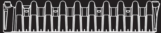
3d. A “push-out” tab is located on the “post end” of each chamber. This tab should be utilized at the end of each trench line run to prevent soil migration from entering the septic system. Press the “push-out” tab over the “post end” lip until it snaps into place.
