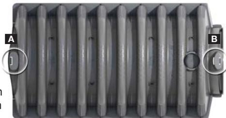
3b. Assemble all Arc chambers in the trench excavation by first placing the “dome end” of the incoming chamber over the “post end” (B) of the chamber already in place. Raise the post end of the incoming chamber and slightly pull the chamber back until the dome stops and is locked into the post end joint.
