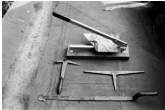
These traditional slater's tools are used to cut and trim, hammer, measure, and rip out nails. Photo: Jeffrey S. Levine.
