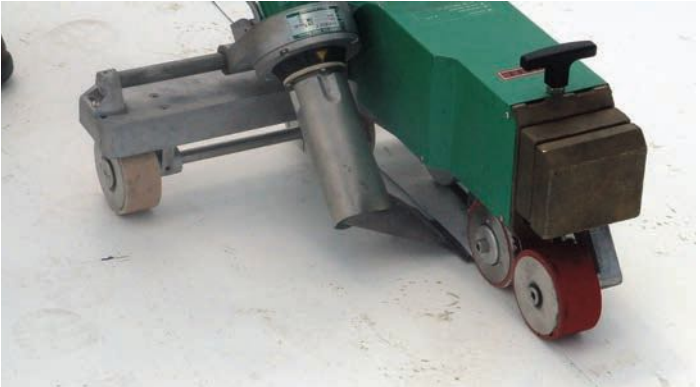
Flex Automatic Hot Air Welding Machine
