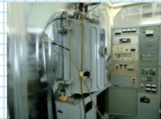
Vacuum deposition equipment
