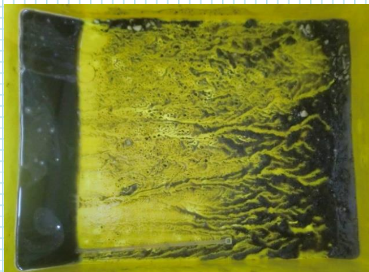
Slurry from the piping passage
