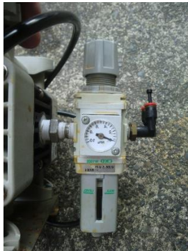
Pump regulator 0.3-0.7Mpa Set to the highest pressure
