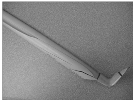
Image 25. Examples of damage resulting from freezing
