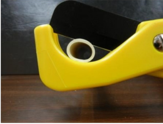
Image 19. Scissor Cutter: not recommended for CPVC
