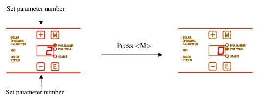
c.) Press the <+> or <-> key to set the selected boiler operating parameter value.
