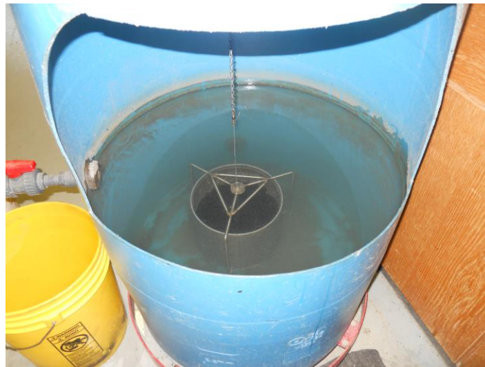
FIGURE 13 Standard maximum theoretical specific gravity test
