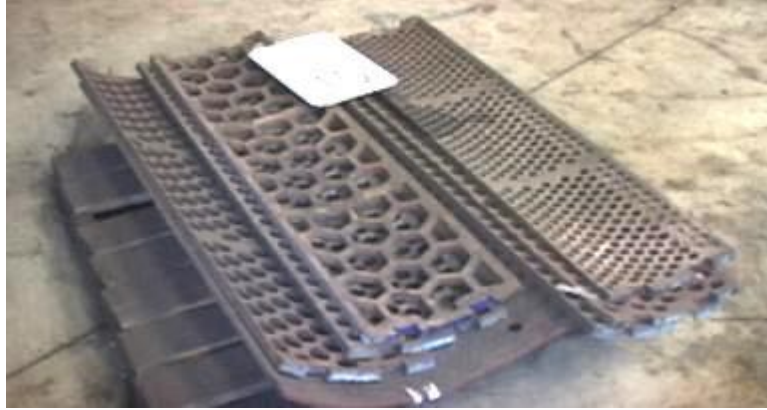
FIGURE 4 Grinding chamber sizing screens (20)
