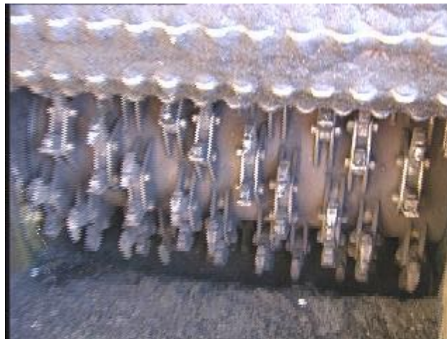
FIGURE 3 Cutting teeth inside grinding chamber (20)
