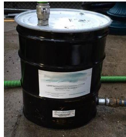
Figure 9. A carbon-filter within this 60-gallon drum is used to remove hydrocarbons and asbestos from water collected in settling tank. Photo courtesy of John Pavitt, US EPA Region 10. No endorsement is implied. Information is included for instructional purposes only.
