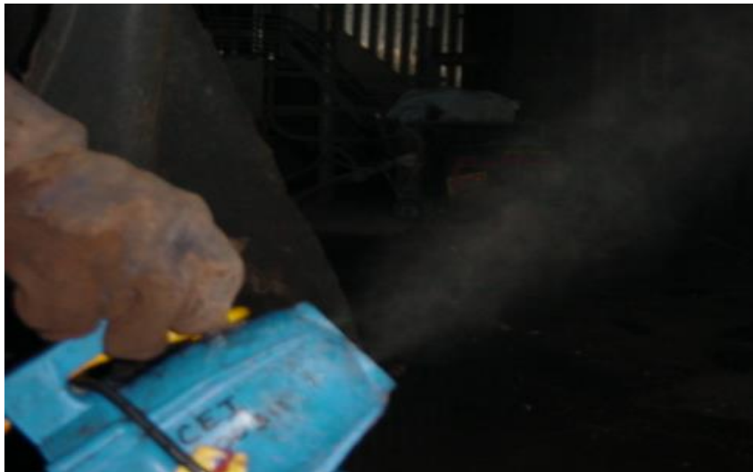
Figure 12. This is an example of one type of low pressure misting nozzle, which is used to suppress and control dust. No endorsement is implied. Information provided for instructional purposes only.
